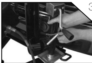
3. Remove crankstand from lift frame.
