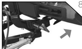
8. Back vehicle away from plow assembly.
