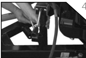
4. Attach crankstand to A-frame.
