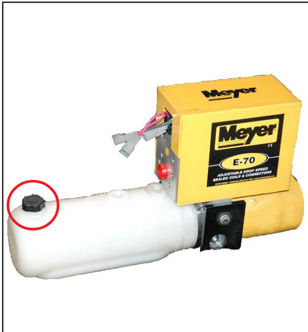
FIGURE 3-72 Fill Hydraulic Unit with Meyer M-1 Fluid. Flush out hoses, lift cylinder and both angle cylinders before operating plow.
