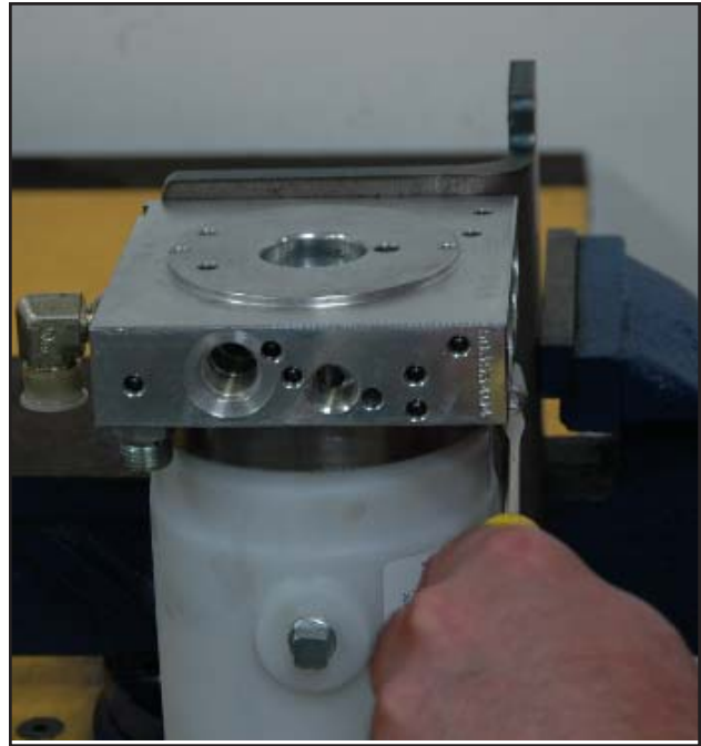
FIGURE 3-51 Clamp reservoir to base with reservoir clamp. Do not use sealant.
