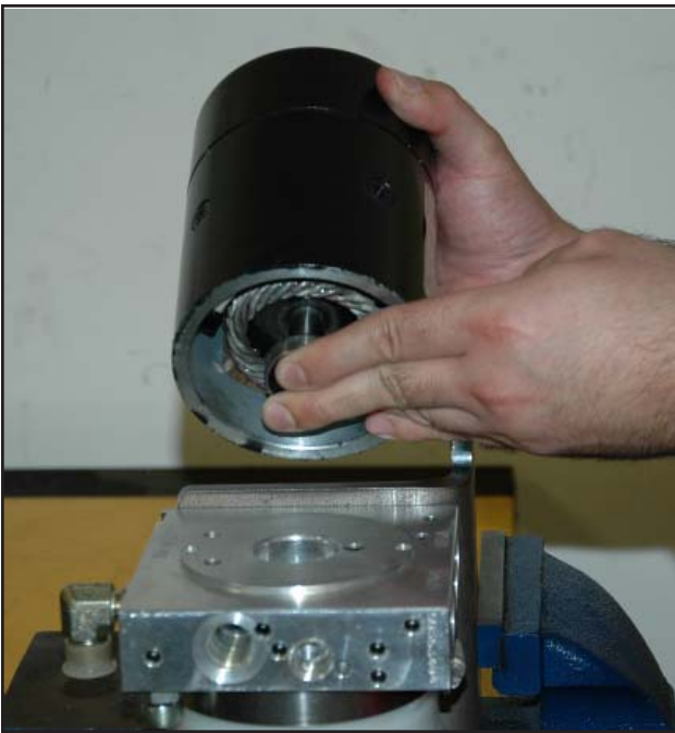
FIGURE 3-52 Carefully re-install motor to base. Be sure motor shaft aligns with pump shaft.
