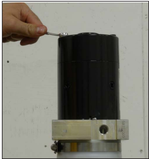
FIGURE 3-53 Tighten motor mounting bolts to base using a 7/16" wrench.
