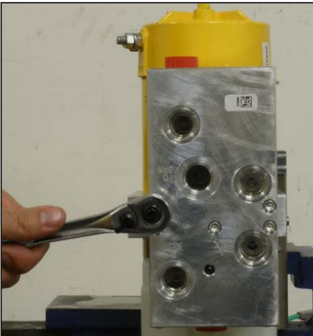
FIGURE 3-28 Use a allen wrench to loosen and remove 4 allen bolts which hold the PA Block to the Base.
