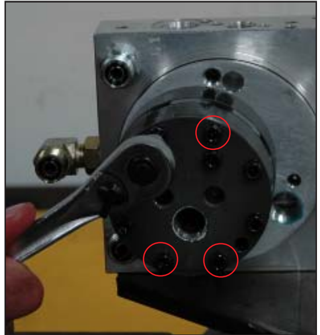
FIGURE 3-39 Use an allen wrench to loosen and remove the 4 bolts holding the pump to the base.
