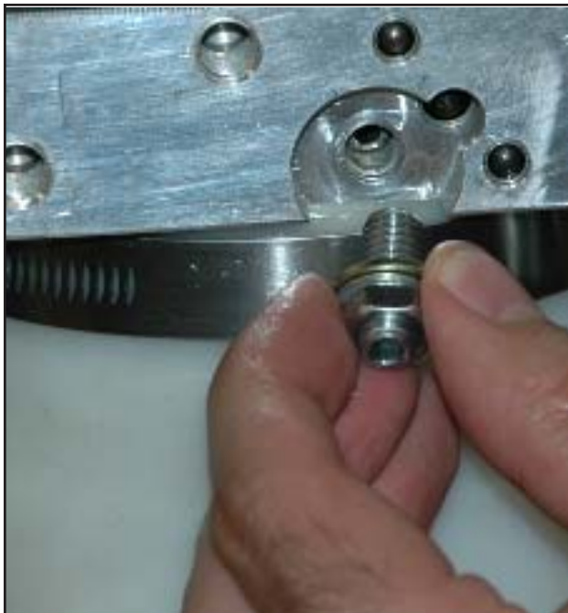
FIGURE 3-56 Install pump relive valve adjuster. This will be adjusted when hydraulic unit is back on plow. Put a guage in an angle hose and extend the angle hose all the way, while holding the button for angle set pressure to 1750 P.S.I. (tighten increases and lossening decreases pressure).
