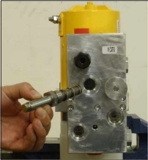
FIGURE 3-66 Re-install "C" Valve
