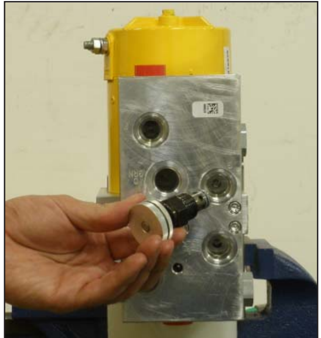
FIGURE 3-63 Re-install Lower Adjustment Assembly. To adjust drop speed of the plow turn the knob in for slower and out for faster drop.
