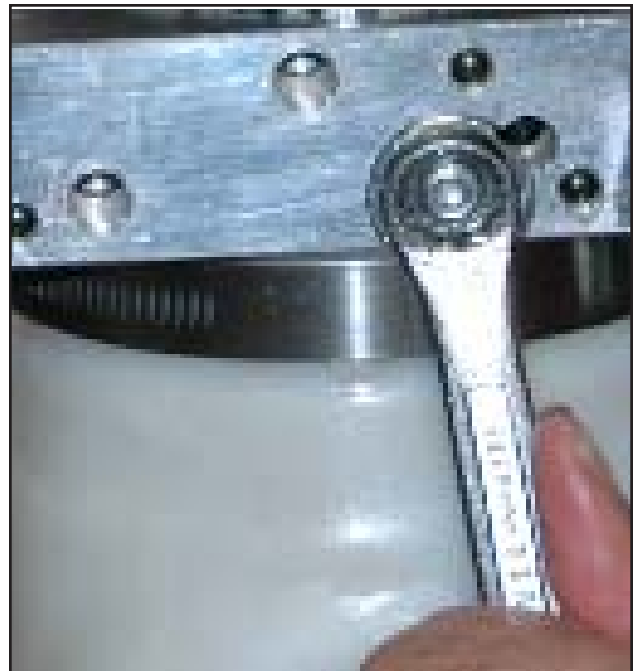
FIGURE 3-57 Tighten adjuster jam nut after pressure has been set to 1750 P.S.I.
