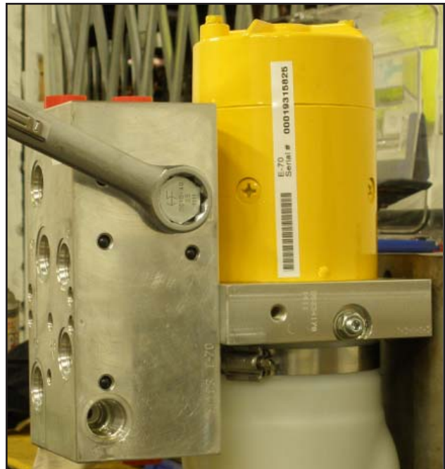
FIGURE 3-21 Use a 1" wrench or socket to loosen and remove Pilot Check Valve Assembly.
